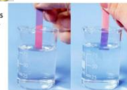
Litmus Paper turns Red when dipped in an Acidic Solution
